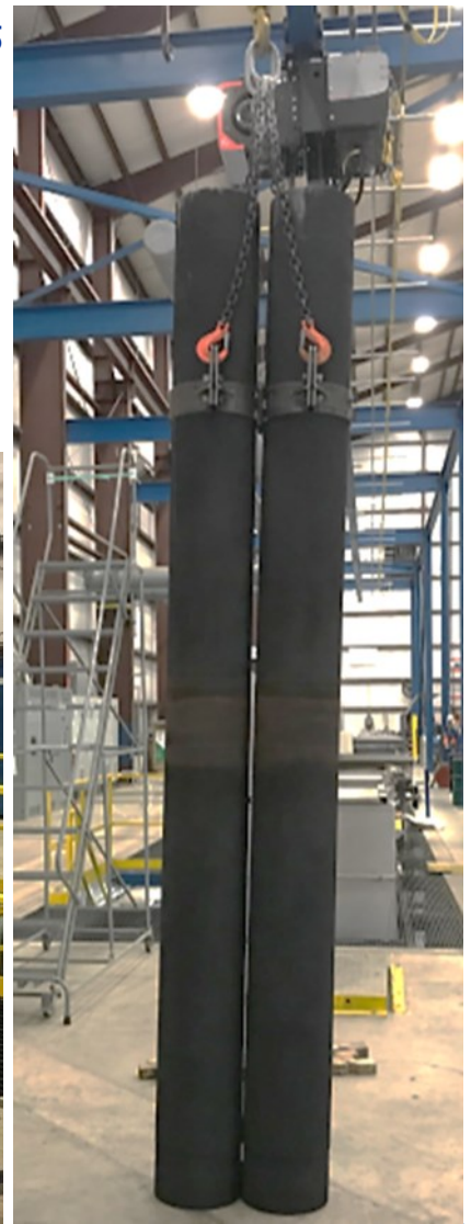
12 feet long, 2000 lb. accumulator tubes
